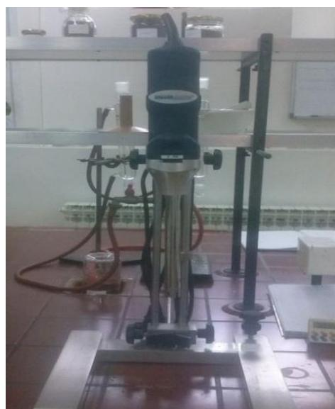
**Slika 5** Homogenizator sustav tip rotor/stator (Izvor: autor)
